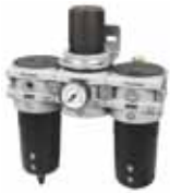
Filter + Regulator + Lubricator Combinations 40 micron element, 12 bar Regulator + Gauge and Wall Mounting Bracket
